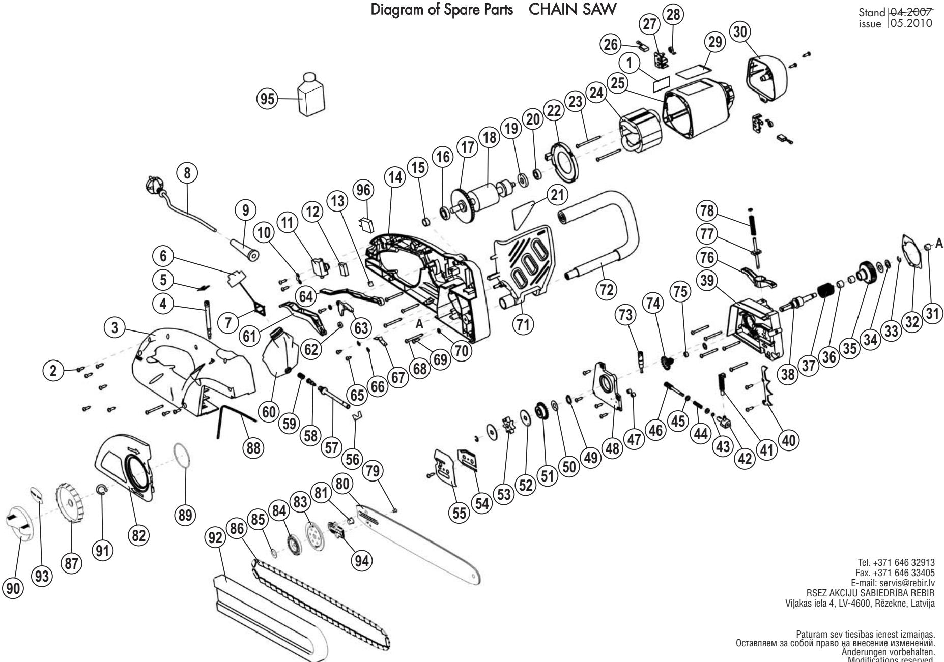
Spare parts supply via REBIR service offices. When ordering spare parts quote power tool type as and date of manufacture. Indicate per machine label, date as per Diagram of Spare Parts, desired spare part number and name as per List of Spare Parts and desired quantity.
